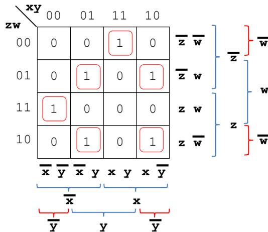
$$f = \bar{x}\bar{y}zw + \bar{x}y\bar{z}w + \bar{x}yz\bar{w} + xy\bar{z}\bar{w} + x\bar{y}\bar{z}w + x\bar{y}z\bar{w} = \bar{x}w(y\oplus z) + y\bar{w}(x\oplus z) + x\bar{y}(z\oplus w)$$
