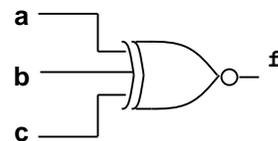
$$f = \overline{\overline{a} \overline{b} \overline{c} + \overline{a} b \overline{c} + a \overline{b} \overline{c} + a \overline{b} c} = \overline{\overline{a}(\overline{b} \overline{c} + b \overline{c}) + a(\overline{b} \overline{c} + \overline{b} c)} = \overline{\overline{a}(b \oplus c) + a(b \oplus c)} = \overline{a \oplus (b \oplus c)} = \overline{a \oplus b \oplus c}$$
